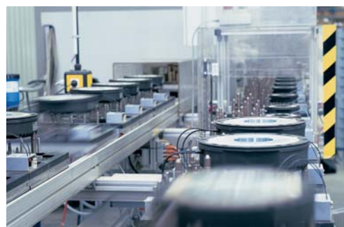
LEFT: FLEXIBLE ASSEMBLY SYSTEM, CAPACITY 1000 MIXED BRAKES PER SHIFT.
