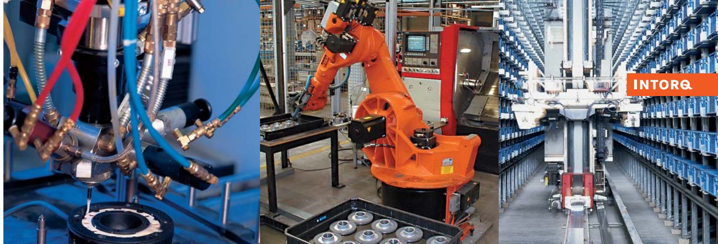
FROM LEFT TO RIGHT: CNC CASTING SYSTEM, ROBOT-CONTROLLED MACHINING OF FRICTION LININGS, AUTOMATIC SMALL PARTS STORE.
