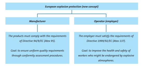
The European Atex Directive has been in force since July 1 2003; it regulates the use of equipment in potentially explosive atmospheres.
