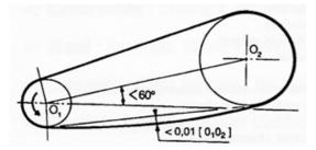
Where the angle of inclination exceeds  $60^{\circ}$ , and where a vertical drive cannot be avoided, precautions must be taken to ensure proper chain-to-sprocket gearing on the power sprocket.
