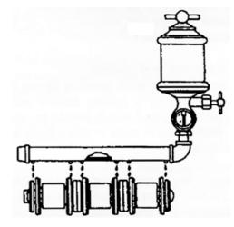
The operator must achieve a compromise between a low viscosity lubricant which would centrifuge off the chain with properly lubricating it, and a substance with too high a viscosity, which would prevent the lubricant reaching contacting surfaces.
